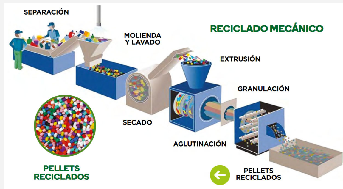
FIGURE 19 Mechanical recycling process
